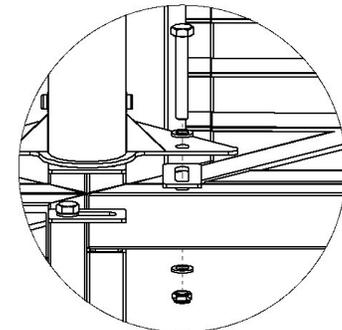
*Aluminum:* Install Hex Head Screws with Flat Washers above and Flat Washers with Lock Nuts underneath. Fully tighten with Wrenches (8 places).
