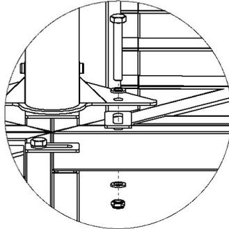
*Aluminum:* Install Hex Head Screws with Flat Washers above and Flat Washers with Lock Nuts underneath. Fully tighten with Wrenches (5 places).
