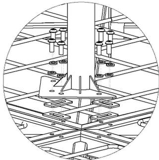
*Stainless Steel:* Install Socket Head Cap Screws with Lock Washers. Fully tighten with Hex Key (8 places).
