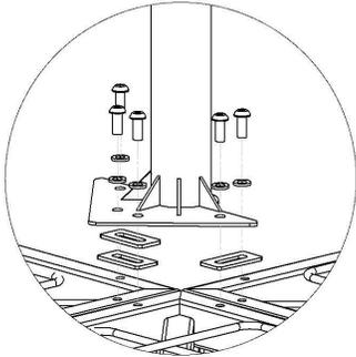
*Stainless Steel:* Install Socket Head Cap Screws with Lock Washers. Fully tighten with Hex Key (5 places).
