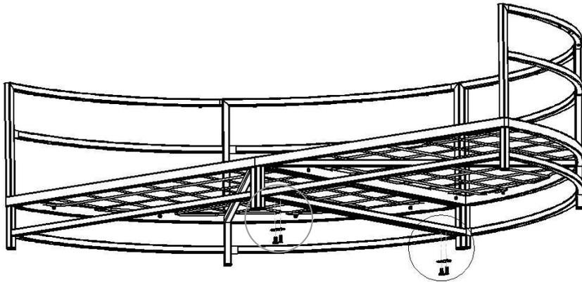
Repeat to attach the 3<sup>rd</sup> and 4<sup>th</sup> sections if these are components are part of the configuration. All section junctions should be retained with two (2) Connector Plates on the bottom of the furniture.
