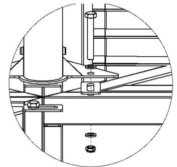
**Stainless Steel:** Install Pan Head Screws with Lock Washers. Fully tighten with Hex Key (4 places).
