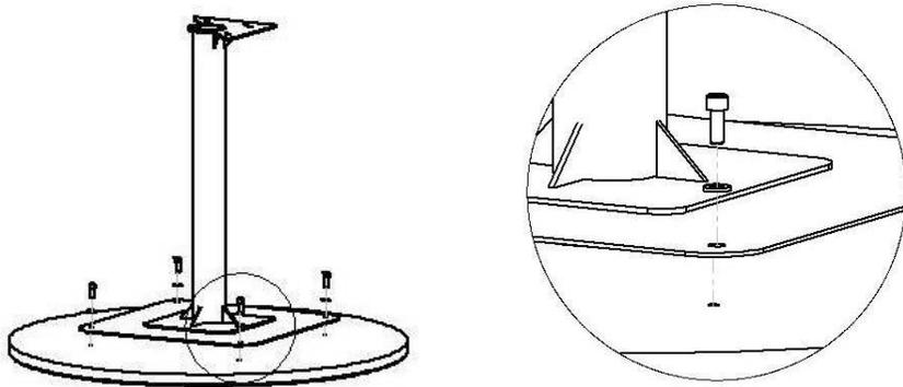
Fully tighten all screws using the Hex Key (4 places).
