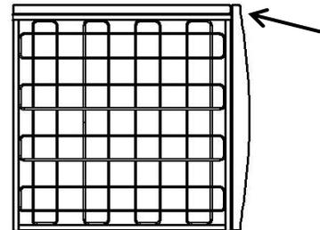
Radius panels overhang the end of the module to form a butt joint with the Flat panel making a finished seam.
