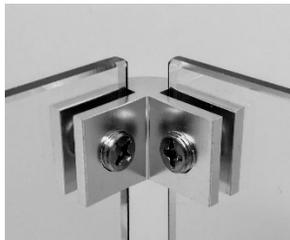
With the Upper Bracket Assembly Screw holes facing inward, slide the Upper Bracket over two joining Glass Panes. Lightly tighten the Set Screw with plastic nib to secure the Glass Panes with the Upper Bracket. DO NOT over tighten the screws. Over tightening may cause the glass to break.
