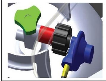
First turn the LP Gas tank (if installed) fully off by rotating the valve completely to the left until closed. Then disconnect the LP Gas tank hose with built in regulator by turning the large connector fully counter-clockwise until the hose is completely disconnected.
